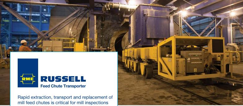
plus maintenance and is vital for fast relining. When a problem or delay is encountered, it can impact maintenance efficiency, plant floor structural integrity and mill availability. Built to work hard over the long haul, **RUSSELL Feed Chute Transporters (FCTs)** allow even the most fully choked loads to be handled with ease, speed and safety.
