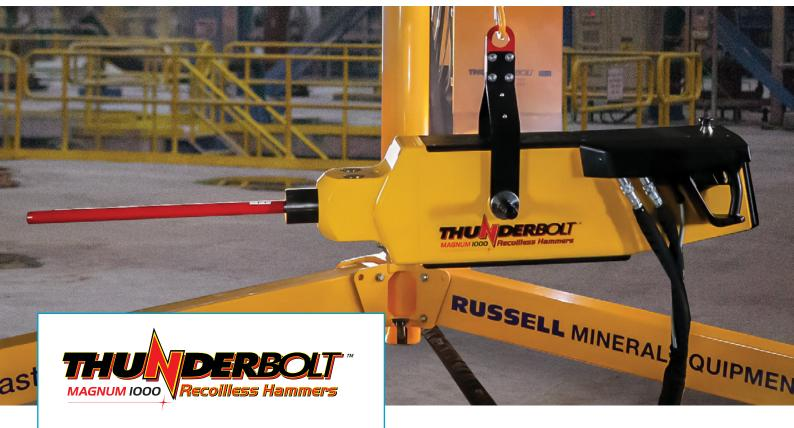
The **THUNDERBOLT** *MAGNUM* **1000** is the industry's most productive recoilless hammer yet. Its impressive, accelerated strike rate and high velocity rapid fire is proven to shorten the critical knock-in phase during mill relines. The THUNDERBOLT *MAGNUM* 1000's versatile productivity will excel in a wide range of environments and deliver increased mill availability through fast, reliable and safe relines.
