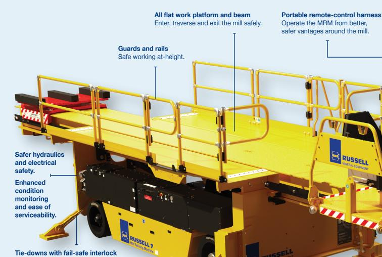
**Tie-downs with fail-safe interlock** Anchor your MRM securely ready for heavy-duty lifting.
