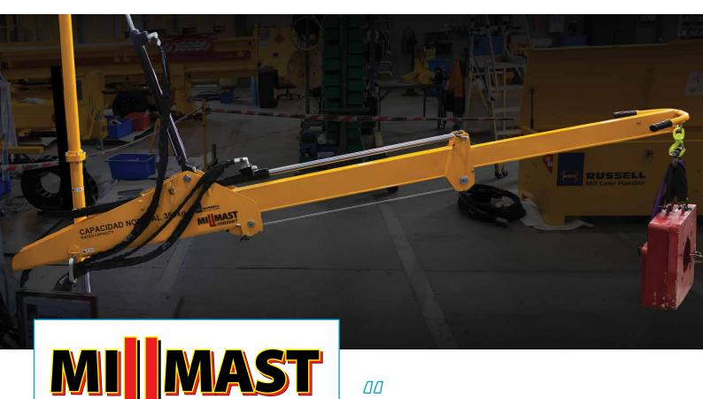
MILLMAST Powershift is a compact mill liner handler tailor-made for smaller space-constrained mills, especially those still wrestling with manual relining. Simple set up and operation, robustlybuilt to handle liners up to 300kg, MILLMAST Powershift prioritises crew safety by reducing manual liner lifting risks and accelerating relining speed. Tough and fatiguing relines in tight spots can be a thing of the past. Let MILLMAST Powershift handle the heavy lifting.
