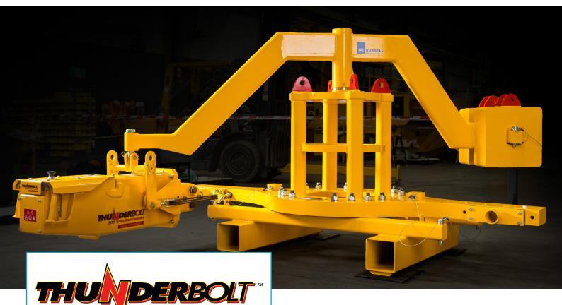
The **THUNDERBOLT Orbit™** all-in-one solution is a literal revolution for cone crusher mantle liner change outs. By delivering high-velocity blows from a THUNDERBOLT Recoilless Hammer, it releases worn mantle nuts and easily secures replacements. The THUNDERBOLT Orbit eliminates the need for human force and represents the fastest and safest method for mantle nut removal and tensioning.
