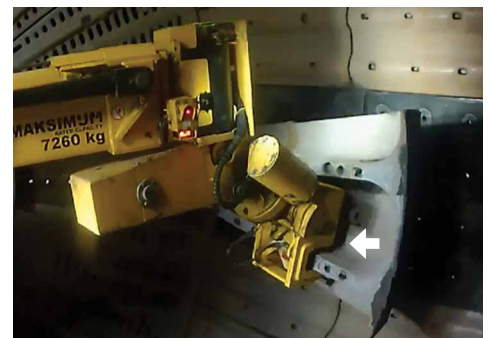
INSIDEOUT PulpXchange Tool removing Bradken pulp lifters
