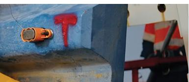
The BOLTBOSS magnetic retention system securely holds liner bolts during the liner placement process, allowing the liner bolt to be pulled through from outside the mill.
